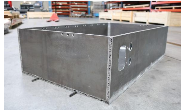
Customized battery box with integrates cooling pipes
