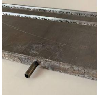
closed cell aluminum foam with open porous structure on one side
