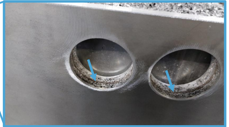
Aluminum foam sandwich (AAS 20-2-2) with an 1mm aluminum-/silicon oxide fiber sheet, customized manufacturing
