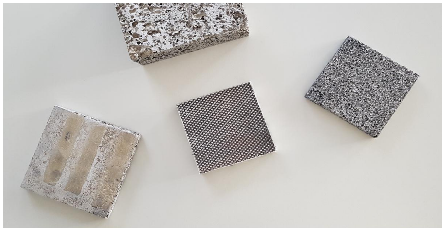
Pure aluminum foam panel with cast skin as outer layer
