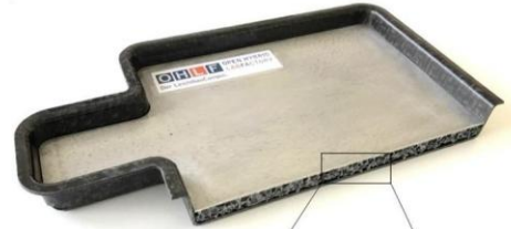
closed cell aluminum foam with open porous structure on one side
