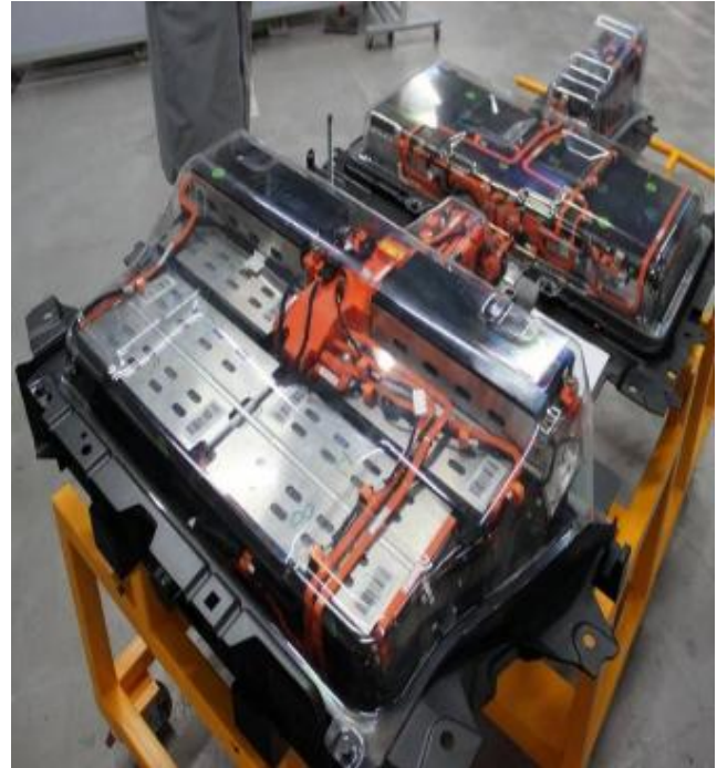
Battery pack of an EV with cooling plates between modules
