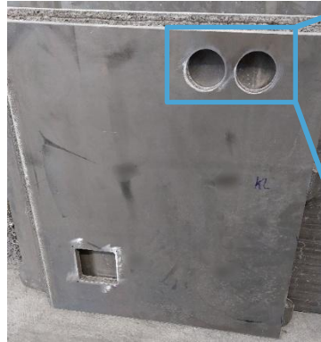
Aluminum foam sandwich (AAS 20-2-2) with an 1mm aluminum-/silicon oxide fiber sheet, customized manufacturing
