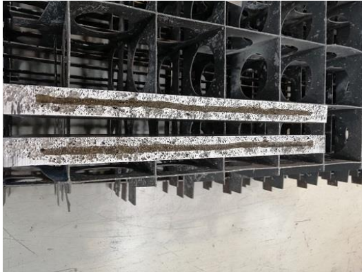
20mm aluminum foam with 6mm rock wool insulation
